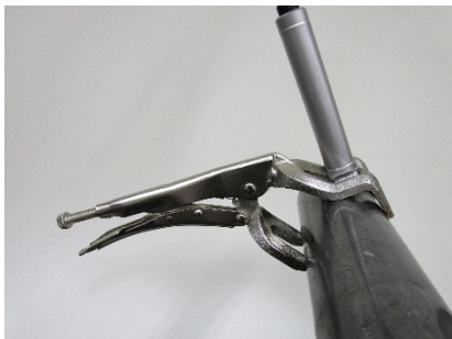
clamp the jaw locking pliers
