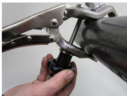
to release the locking spindle again, the pliers should be clamped
