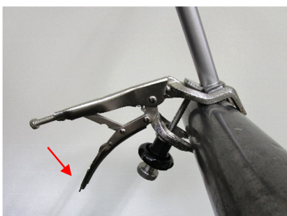
clamping holds reliably, even when the tongs are released
