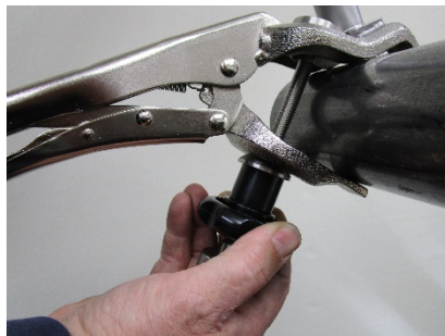
turn the clamping cone tightly with the black handwheel
