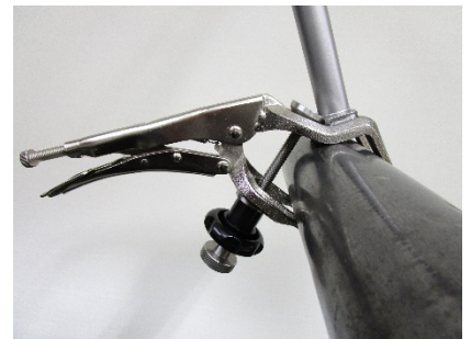
until the jaws are jammed - now the gripper is secured against rotation
