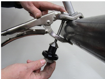
insert threaded rod from below and tighten with locking wheel*
